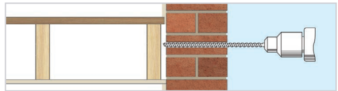
1. Mark the position of the joist centre on the external wall and then drill a clearance hole (normally \frac{5}{8} " ) through the wall. Clean out the hole
