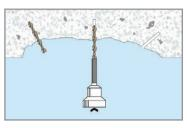
3. Fit the PatchPin drill sleeve driver over the drill bit and insert the PatchPin into the tool. Install the PatchPin into the pilot hole with the SDS rotary hammer drill set to hammer only. Ensure that the outer end of the pin will be below the face of the concrete patch – the pin can be bent, if required.
