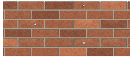
1. Install wall ties both sides of the intended vertical movement joint in a grid pattern
