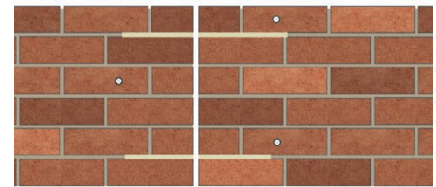
2. Cut horizontal slots in the mortar beds. Cut the vertical movement joint
